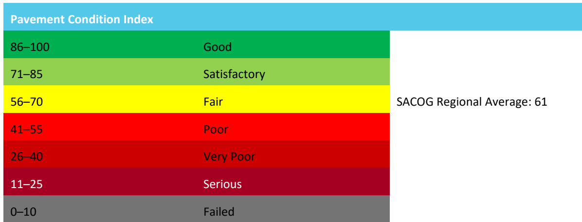
FIGURE 4.8 PAVEMENT CONDITION INDEX
